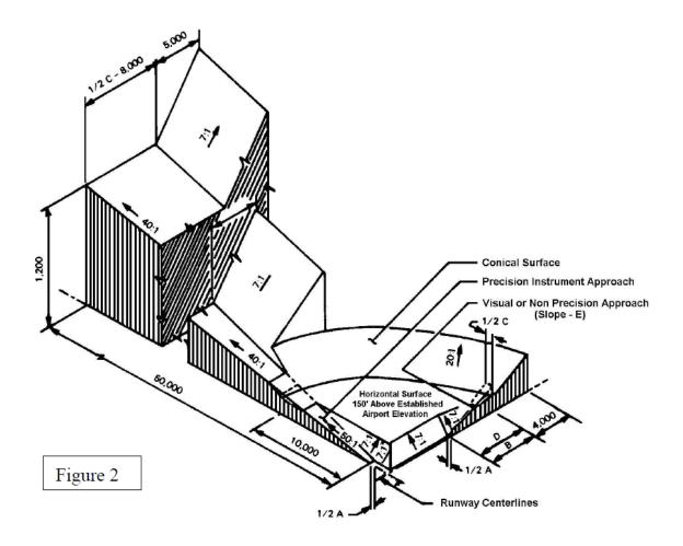
Source: NOAA National Geodetic Survey, FAA 3D-Diagram of FAR Part-77 Surfaces
