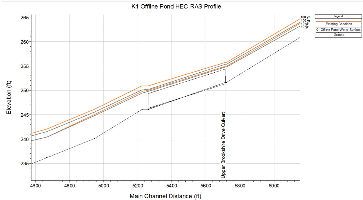
Figure #: 10-yr and 100-yr Water Surface Profile on Upper K1 with Offline Pond
